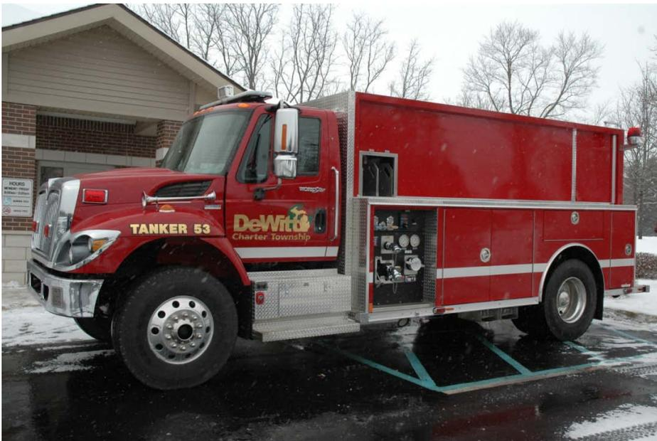
On January 7, 2011, the DeWitt Township Fire Department took delivery of a new water tanker. This vehicle, on an International chassis, will replace a 1985 GMC water tanker. While this vehicle is a little smaller than the previous tanker, it is more maneuverable and has more capabilities. This vehicle carries 2,100 gallons of water and has a 500 gallon per minute pump. This purchase is part of a long-term vehicle replacement plan adopted by the Township's Board of Trustees.
